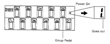
When the FC-100mk II is set to the RRC Foot Pedal mode, the Point  ${\rm 1\!\! I}$  will go out.
