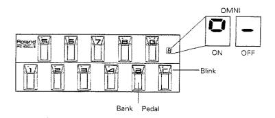
2) Press the Control Pedal 9, then go to step 4.
