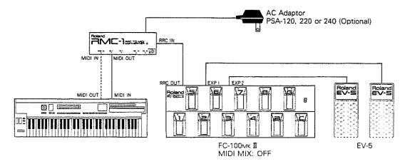
The FC-100mk II can crontrol a sound module or keyboard. If you connect the MIDI OUT socket on the external instrument to the MIDI IN on the RMC-1, the display of the FC-100mk II will match that of the external device. (Set the FC-100mk II to MIDI MIX Off as explained in the following section.)
