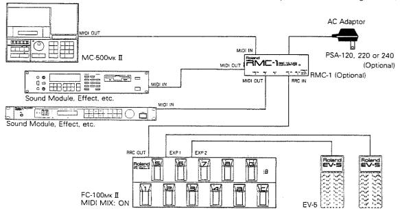
The FC-100mk II can also control a sound module that is at the same time being controlled by a sequencer. (Set the FC-100mk II to MIDI MIX On as explained in the following section.)
