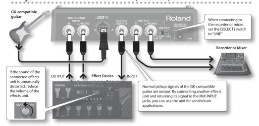
\* When connection cables with resistors are used, the volume level of equipment connected to the inputs (MIX/GUITAR INPUT jacks) may be low. If this happens, use connection cables that do not contain resistors.
