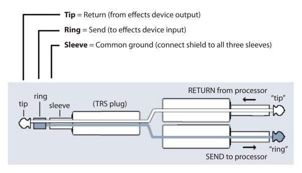
The master effects loop allows all three guitars (guitar synth input, auxiliary input 1, and auxiliary input 2) to be processed at the same time, through external effects.
