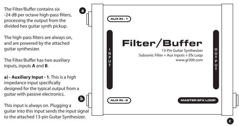
While this input is designed for guitar signals, it can be used with any audio source. This input is a tip-sleeve, unbalanced input.
