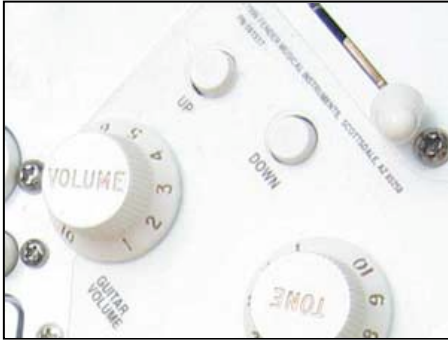
The industry-standard Fender Roland-Ready Strat uses two momentary push buttons for GK S1 and S2 switch, here labeled Up and Down .
