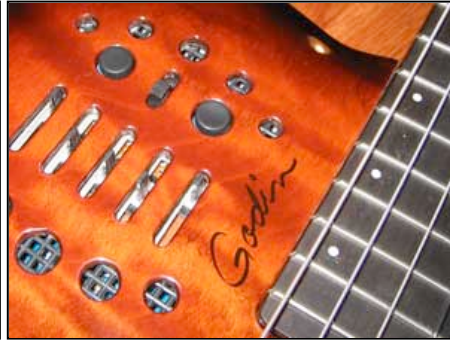
Similar to the Fender Roland-Ready guitar, Godin has two momentary pushbuttons for S1 and S2.
