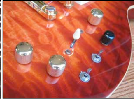
S1 and S2 are combined on one spring loaded toggle switch on the Brian Moore Roland-Ready guitars.
