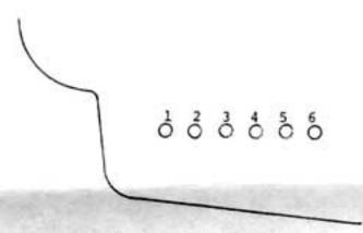
Insert screw driver into holes on back of guitar, turn clockwise to increase sensitivity.
