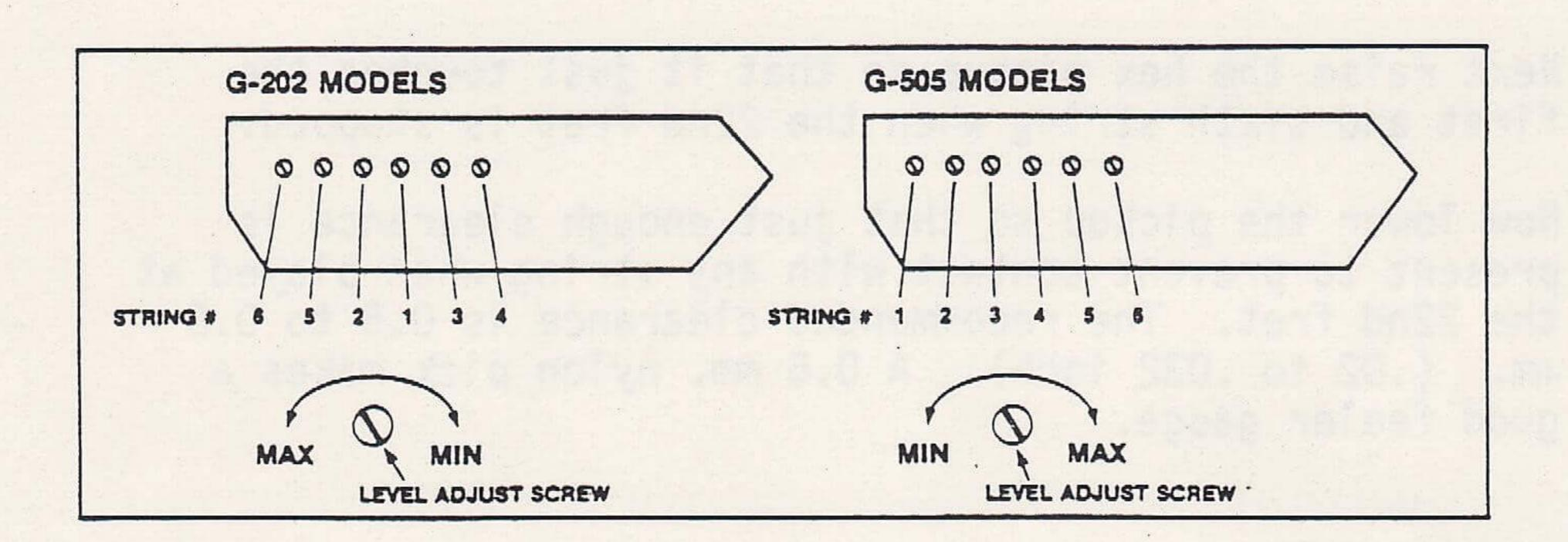
Check that the controls for all strings are set at approximately mid-rotation to start. (This is the way they are generally set at the factory.)
